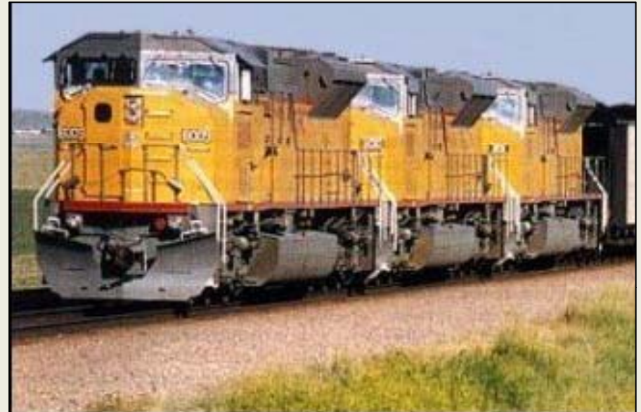
Three of the new 6,000 hp US diesel-electric locomotives
